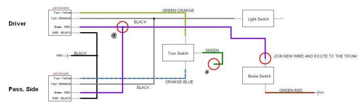
@ TEE INTO NEW WIRE AND CONNECT TO SECOND LED UNIT
