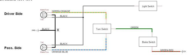
X ON 64-65 THE BULBS ARE GROUNDED DIRECTLY THROUGH THE LIGHT HOUSINGS AND THIS CONNECTION DOES NOT EXIST
